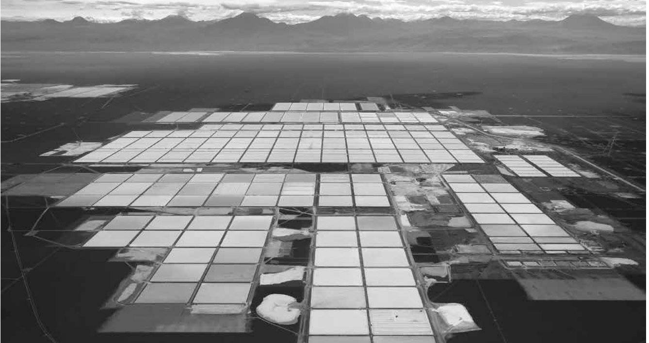
Lithium brine evaporation on the Salar de Atacama, Chile
